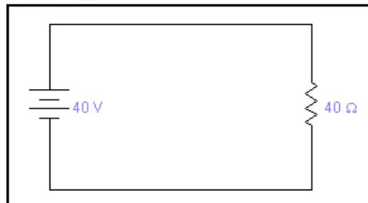
The current flowing through 40 ohm resistor by Ohm's law is
