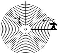
Moving observer, source at rest. If the observer was at rest, the number of waves she would receive in time t would be t/T (or  $vt/\lambda$ ). But if she is moving towards the source with speed v<sub>0</sub> (as in the above figure), the additional number of waves received is obviously  $v_0 t / \lambda$ . By definition,
