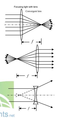
12. Here is how a concave (or divergent) lens forms an image. An observer on the side opposite to the object will see the image upright and smaller in size than the object.
