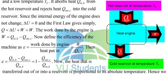
arrive at the important result that  $\varepsilon = 1 - \frac{T_c}{T_c}$ . This number is always less than one, showing that no machine can convert all the input heat into useful work. As an example, a nuclear reactor has temperature  $300^{\circ}C$  at the core and rejects heat into a river at  $30^{\circ}C$ . The maximum efficiency it can have is  $\varepsilon = 1 - \frac{30 + 273}{300 + 273} = 0.471$
