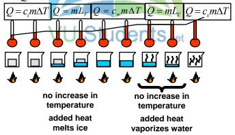
In the above diagram you see what happens as ice is heated. The amount of heat needed is indicated as well. Note that no change of temperature happens until the phase change is completed. The same physical situation is represented to the right as well where the temperature is plotted against Q.
