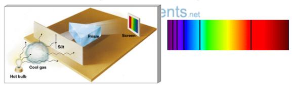
The above shows the absorption spectrum of a certain atom. The wavelengths for both emission and absorption lines are exactly equal. Classical physics and the Rutherford model have no explanation for the spectrum.
