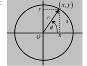
2. The arc length = radius  $\times$  angular displacement, or  $s=r\phi$ . Here  $\phi$  is measured in radians. The maximum value of  $\phi$  is
