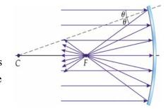
7. The concave mirror is different. A parallel beam incident from the left is reflected and the rays now spread out (diverge). However, if we were to look at any outgoing ray and extend it backward, all the rays would appear to be coming from one single point. This is the *virtual focus* because there is, in fact, no real source of light there. From the diagram you can see the virtual focus F is at distance R/2 behind the mirror. We say that the focal length of such a mirror is f = -R/2.
