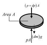
Note that we are taking the origin (y = 0) at the bottom of the liquid. Therefore as the elevation increases (dy) positive, the pressure decreases (dp) negative. The quantity  $\rho g$  is the weight per unit volume of the fluid. For liquids, which are nearly incompressible,  $\rho$  is practically constant.
