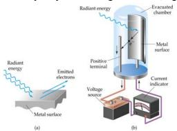
and knocks out electrons that travel to the anode. A current flows only as long as the light is shining. Above the threshold frequency, the number of electrons ejected depends on the intensity of the light. This was called the photoelectric effect. The following was observed:
