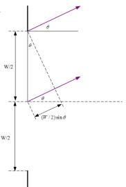
9. Light with wavelength of 511 nm forms a diffraction pattern after passing through a single slit of width 2.2×10<sup>-6</sup>m. Find the angle associated with second bright fringe above the central bright fringe.
