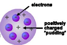
5. But the plum-pudding model was wrong. In 1911, Rutherford carried out his famous experiment that showed the existence of a small but very heavy core of the atom. He arranged for a beam of  $\alpha$  particles to strike gold atoms in a thin foil of gold.
