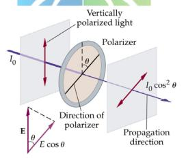
Each wave is reduced in amplitude by  $\cos \theta$ , and in intensity by  $\cos^2 \theta$ . The wave that emerges is now polarized in the  $\theta$  direction.
