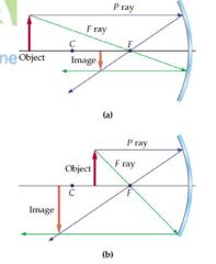
9. Now repeat for a concave mirror. Here the rays will never actually meet so we can have only a virtual object. Take 3 rays - call them P,F, and C - and see how they are reflected from the mirror's surface. Where they meet is the position of the image. The image is always smaller than the actual size of the object. This is obviously useful for driving a car because you can see a wide area.
