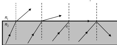
8. Fibre optic cables, which are now common everywhere, make use of the total internal reflection principle to carry light. Here is what a fibre optic cable looks like from inside:
