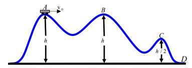
Even though the motion is complicated, we can use the fact that the total energy is a constant to get the speeds at the points B,C,D:
