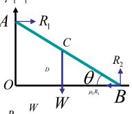
This gives  $\cos\theta \left(R_2 - \frac{W}{2}\right) = \mu_2 R_2 \sin\theta$  from which  $\tan\theta = \frac{R_2 - \frac{W}{2}}{\mu_2 R_2}$  with  $R_2 = \frac{W}{\left(1 + \mu_1 \mu_2\right)}$ .
