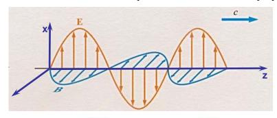
In the diagram above, an electromagnetic wave is moving in the z direction. The electric field is in the x direction,  $E_x = E_0 \sin(kz - \omega t)$ , and the magnetic field is perpendicular to it,  $B_y = B_0 \sin(kz - \omega t)$ . Here  $\omega = kc$ . From Maxwell's equations the amplitudes of the two fields are related by  $E_0 = cB_0$ . Note that the two fields are in phase with each other.
