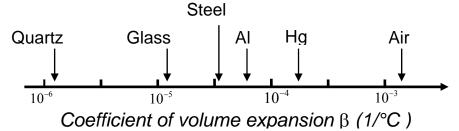
13. We can use the fact that different metals expand at different rates to make thermostats. For example, you need a thermostat to prevent an electric iron from getting too hot or a
