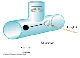
Thus the momentum of the light changes and this creates a force that rotates the mirror. The force is quite small - just  $5 \times 10^{-6}$  Newtons per unit area (in metre<sup>2</sup>) of the mirror.
