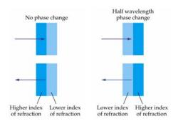
When light falls upon a thin film of soapy water, oil, etc. it is reflected from two surfaces. On the top surface, the reflection is with change of phase by  $\pi$  whereas at the lower surface there is no change of phase. This means that when waves from the two surfaces combine at the detector (your eyes), they will interfere.
