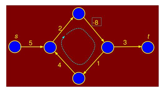
Figure 8.61: Negative weight cycle
