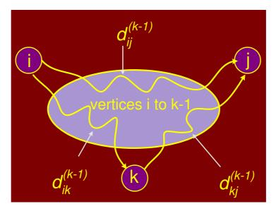
Figure 8.71: Two cases for all-pairs shortest path
