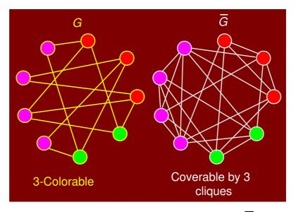
Figure 9.7: 3-colorable G and clique coverable  $(\overline{G},3)$
