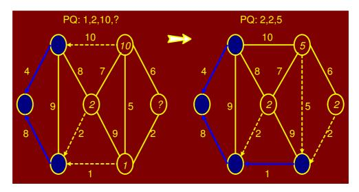
Figure 8.59: Prim's algorithm: edges with weights 8 and 1 selected
