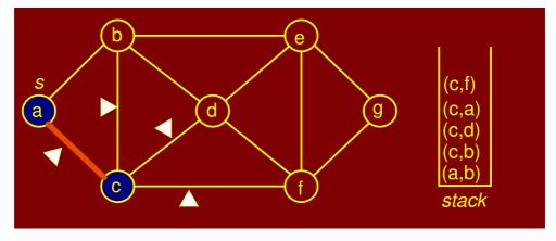
Figure 8.14: Trace of DFS algorithm: vertex 'c' popped
