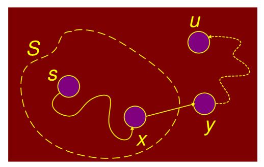
Figure 8.69: Correctness of Dijkstra's algorithm
