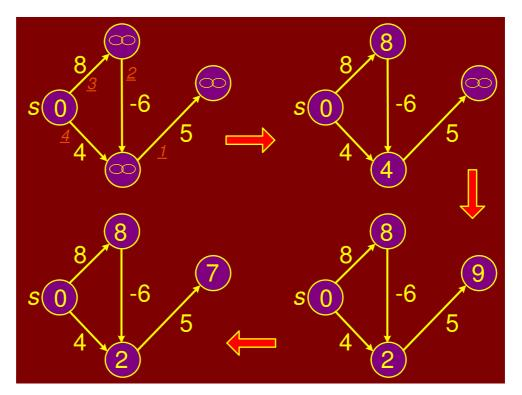
Figure 8.70: The Bellman-Ford algorithm
