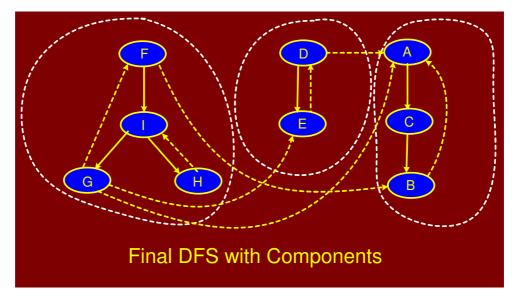
Figure 8.41: Final DFS with strong components of G<sup>T</sup>
