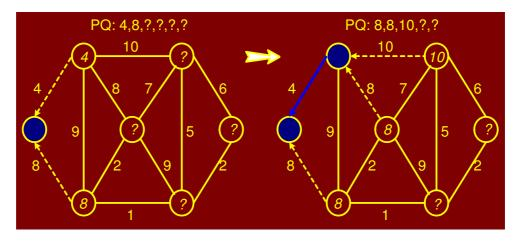
Figure 8.58: Prim's algorithm: edge with weight 4 selected
