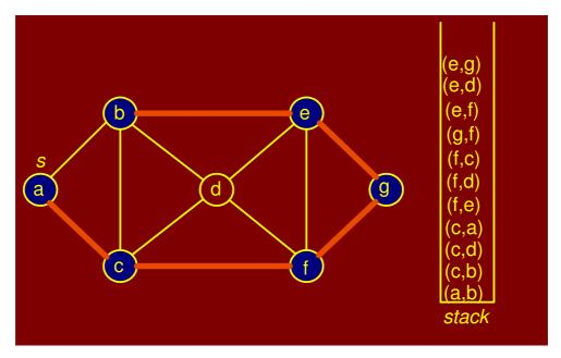
Figure 8.18: Trace of DFS algorithm: vertex 'b' popped
