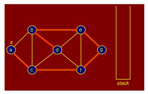
Figure 8.19: Trace of DFS algorithm: vertex 'd' popped
