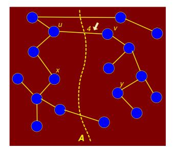
Figure 8.47: MST T which contains light edge (u, v)
