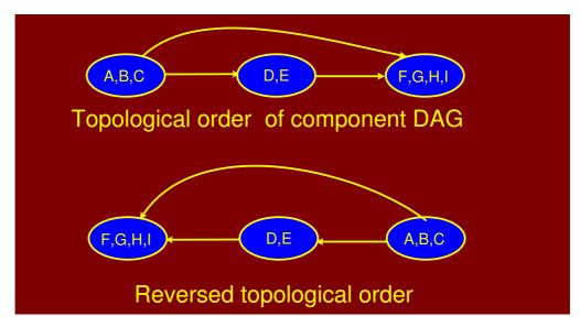
Figure 8.37: Reversed topological sort of component DAG
