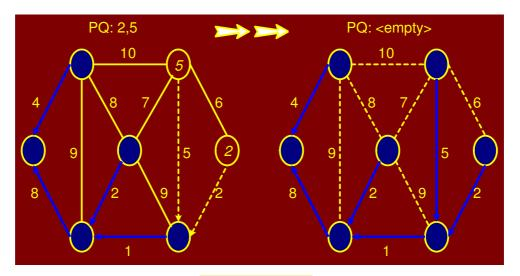
Figure 8.60: Prim's algorithm: the final MST
