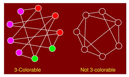
Figure 9.3: Examples of 3-colorable and non-3-colorable graphs
