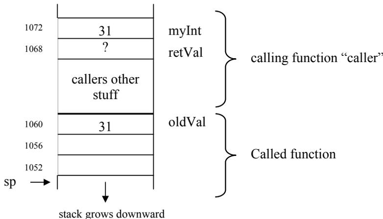
**Fig 17.3:** call stack layout when intMinus1 is called
