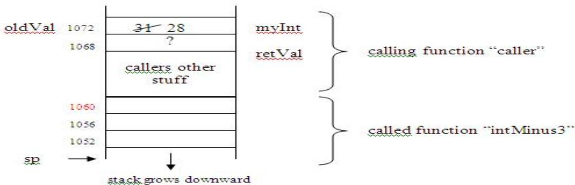
**Fig 17.11:** call stack layout after `oldVal = oldVal - 3 ;`
