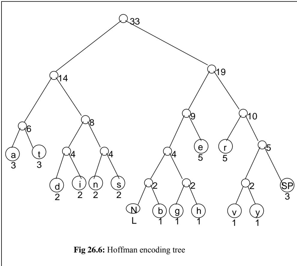
**Fig 26.6:** Hoffman encoding tree
