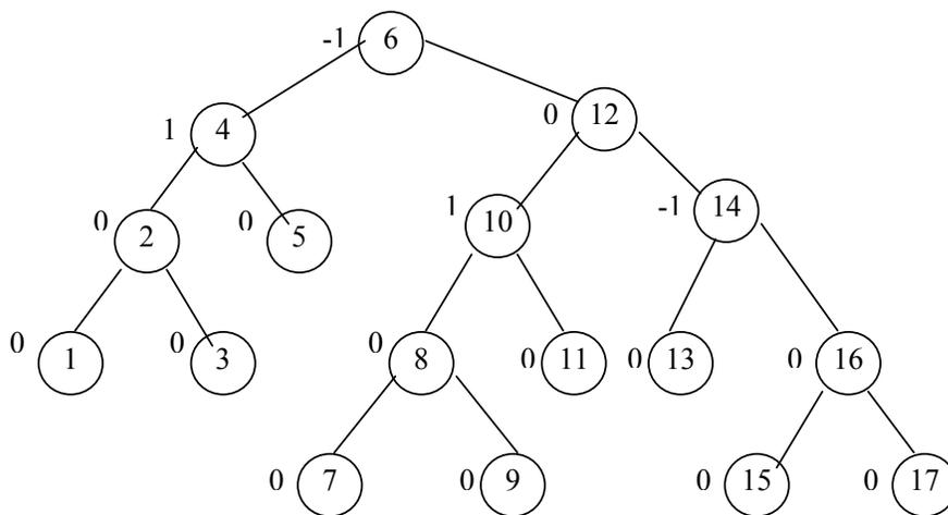
**Fig 20.4:** A balanced binary tree
