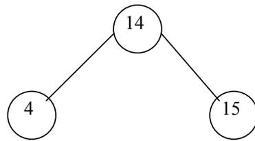
**Fig 13.1:** A three node binary tree
