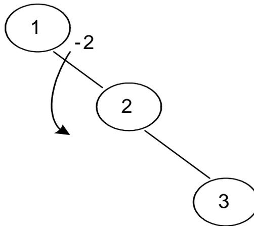
**Fig 21.1: insert(3) single left rotation**
