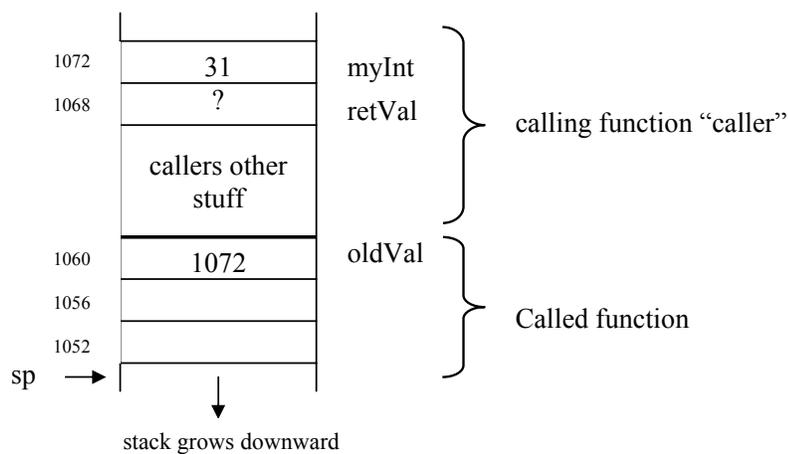
**Fig 17.6** call stack layout when *intMinus2* is called
