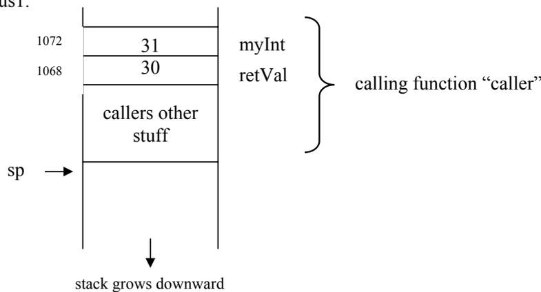
**Fig 17.5** call stack layout after return from *intMinus1*. In the previous function *caller*, we could have called the function *intMinus1* as follows.
