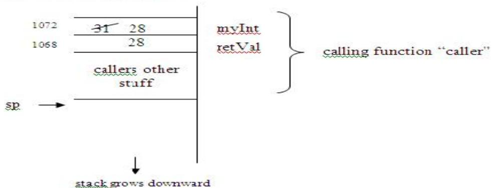
**Fig 17.12:** call stack layout after return from *intMinus3*
